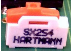
Switch position left (delivery status)
